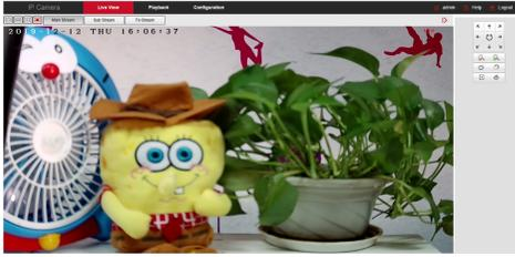
② Click **【Main Stream】** / **【Sub Stream】** / **【Tri-Stream】** to switch the preview stream. Click the corresponding icon in the lower left corner of the interface to stop the live preview, record, capture, and so on.
