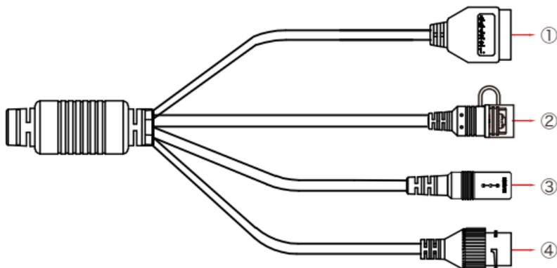
① Alarm interface: including alarm input and alarm output, a group of inputs, a group of outputs and RS485 (used to connect external devices with RS-485 interface).
