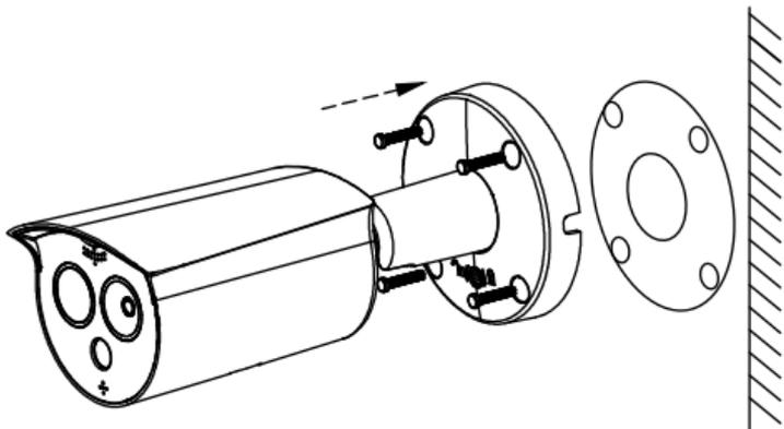
Step 3 Use a hexagon wrench to loosen the fixing screws, then adjust the camera to a proper angle, and tighten the fixing screws to complete the installation.
