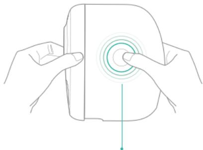
Press buttons on both sides, and pull out the back cover.
