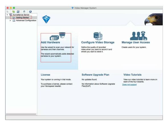
Pop-up dialog box to add add hardware, hardware scans can scan directly inside the LAN hardware device, you can also scan the specified network hardware; manually add the hardware is added directly to know the address or the serial number of hardware devices.
