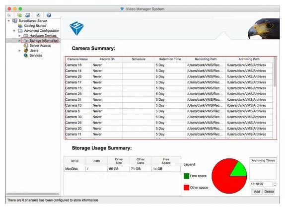
Channel storage configuration editor, double-click to the right of the list box into the recording and storage properties, you can only give one camera configuration can also use templates to configure multiple cameras, (using the template configuration see 2.1.3.3).
