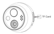
Step 4: Close the TF card cover and tighten the screws.
