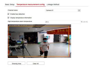
Step 4: Select [Camera 02], draw the bold point (if there is a black body) and reference point, configure related parameters (shutter parameters, temperature compensation, etc.), and click [Save].
