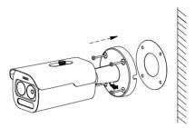
Step 3 Use a hexagon wrench to loosen the fixing screws, then adjust the camera to a proper angle, and tighten the fixing screws to complete the installation.
