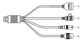
Alarm interface: including alarm input and alarm output, a group of inputs, a group of outputs and RS485 (used to connect external devices with RS-485 interface).
