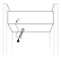
Step 8 Lift the security gate to a vertical position, turn on the power, and the installation is complete.
