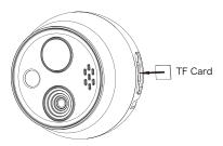
Step 4 Close the TF card cover and tighten the screws.
