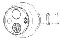
Step 3 Insert the TF card into the card slot slowly, and when you hear a "click" sound, the installation is complete.
