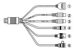
① Alarm interface: including alarm input and alarm output, a group of inputs, a group of outputs and RS485 (used to connect external devices with RS-485 interface).
