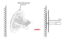
Step 3: Connect wires, install the device on the wall bracket, then align the screw holes on the left and right sides, install the nuts and lock the screws.
