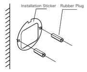
Step 2: Pass the network cable and 10PIN wire through the wall bracket, and arrange the wire into the wire groove, then fix the bracket to the wall with screws.
