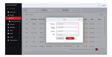
The device is turned on "DHCP" by default after leaving factory.
