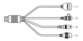
① Alarm interface: including alarm input and alarm output, a group of inputs, a group of outputs and RS485 (used to connect external devices with RS-485 interface).
