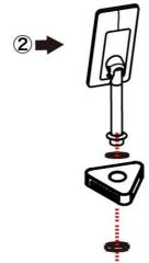
**Step 3:** Pass the wire of the device through the cover, and fix the cover on the bracket with the locking screw.
