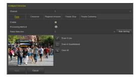
Step 2: Select the smart detection alarm mode for setting the channel. Intelligent detection alarms supported by the device include Face Detection, Crossover Detection, Regional Intrusion Detection, People Stay Detection and People Gathering Detection. Each smart detection can be configured with different alarm rules.
