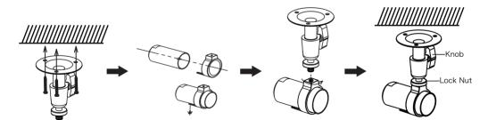
Fix the lens mount 2 to the wall with screws. (2) Insert the pen-shaped lens into the bracket ring and lock it with the screw to ensure that the " ➡ " mark on the lens is directly above. (3) Align the lens threaded port with the lens mount 2 thread and turn it clockwise to secure it to the bracket. (4) Connect the lens cable, compare the image on the monitor to adjust the angle of the lens, and lock the nut and the konb to complete the installation.
